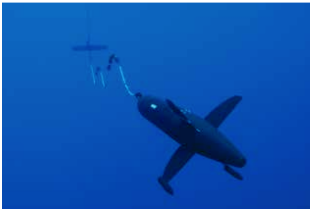
Massive Towing Capability — Tow cable assembly attached to Wave Glider sub
